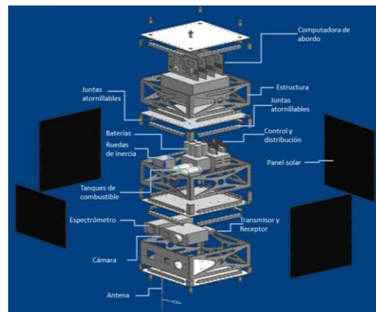
Figure 5 Satellite *Quetzal* First design. There still an ongoing revision of the scientific payload for reducing its size and energy budget.
