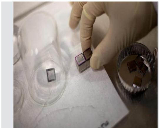
*Figure 3 A pair of mini ion thrusters, including their propellant tanks, is prepared for tests. Credit: M. Scott Brauer Science Daily, taken from Lozano et all*
