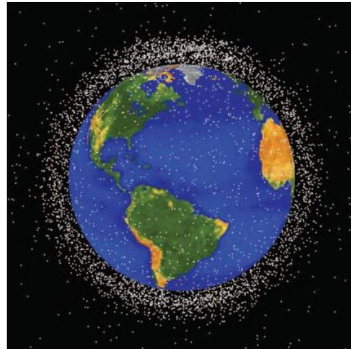
Figure 2 Computer-generated image of objects in low earth orbit that are currently being tracked. Only about 5 percent of these objects are functional satellites; the rest is debris. (The dots are not drawn to scale with Earth.) Credits nasa.gov
