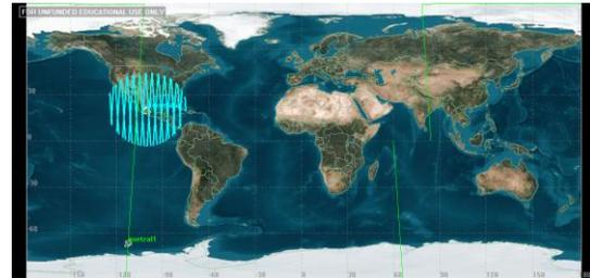
Figure 4 Orbit simulation for the *Quetzal* mission at 600 kms height over Mexican territory
